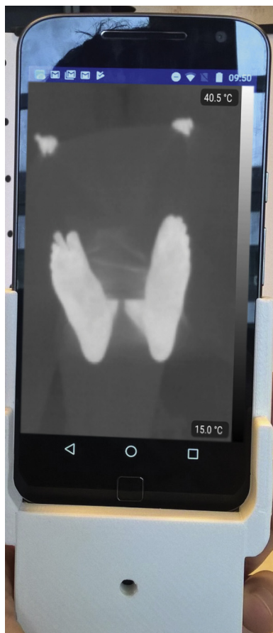
Fig. 1 – Smartphone with underneath a FLIR One IR-camera connected. They are placed within the 3D printed mount for tripod fixation. On the screen is a thermal infrared foot image visible of a participant while holding a black cloth.
